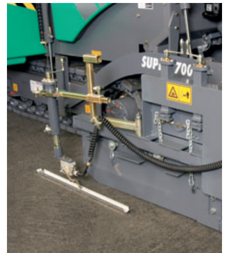
1 Referencing with mechanical grade sensor and ski.
