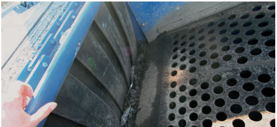
Chains and rubber curtain in use in the MR 130 R EVO impact crusher
